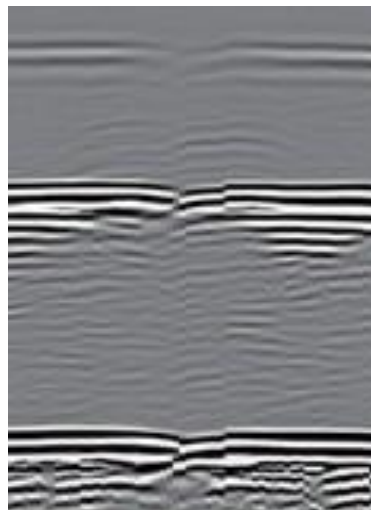
Figure B2.3(a) Through-wall Flaws
